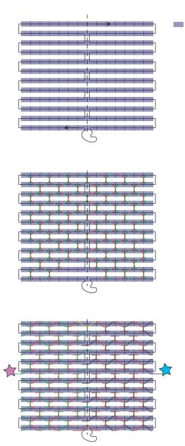
One building block (bb) height: 2 nm length: 16 nt => 1.5 turns => 5.4 nm nt = nucleotide (A, T, G, C base)
